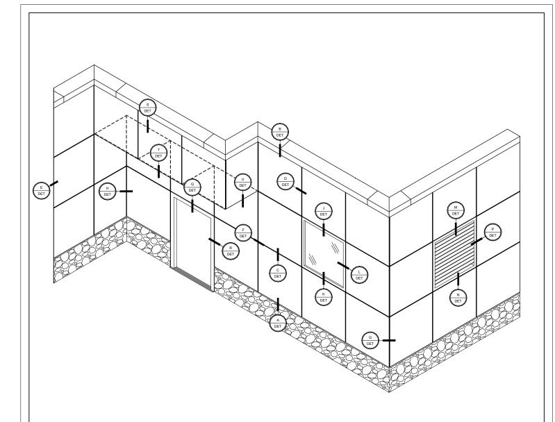
Extruded aluminum furring must be attached to structural members designed to support the dead and live loading of the entire wall system. the following details do not specify, suggest, or imply the attachment between the structure and aluminum furring. The customer is responsible for the structural engineering of attachment to structure.
