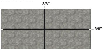
Maintain a minimum distance of 3/8" between panels to accommodate hygrothermal movement of the panels.
